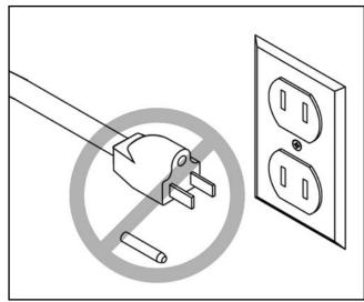
Figure 1A. Do not remove grounding pin.
